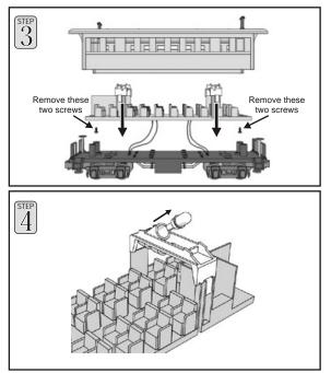
3) To be able to separate the interior from the shell you need to remove the screws from underneath the interior. With the two screws removed you can then lower the interior down from the shell.
