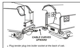
• Connect the draw bar between the engine and tender.
