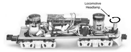
Figure 8. Location of the headlamp in the Engine.
