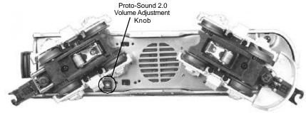
Figure 4. Location of the Proto-Sound 2 Volume Adjustment Knob
