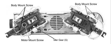
Figure 6. Body Mount Screws and Greasing Points.
