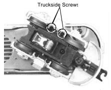
Figure 7. Screws to Remove to Access the Traction Tires
