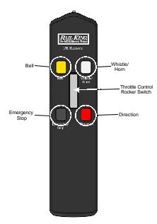
Fig. 3: Overview of the Remote controls
