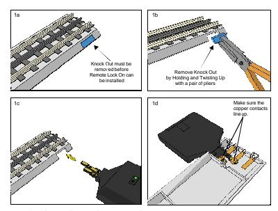
Fig. 1a-1d: Installation of Remote Lock On
