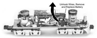
Figure 10. Removing and Replacing the Battery
