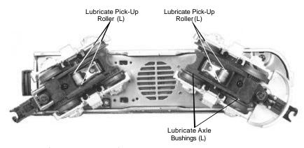
Figure 5. Lubrication Points on the Engine
