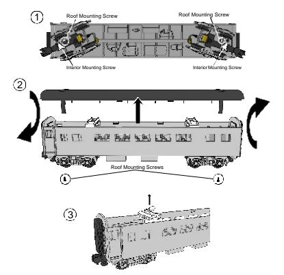
Figure 9. Instructions for Replacing the Lights in the Passenger cars.
