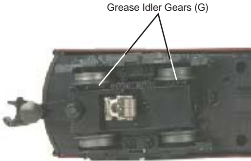
Figure 5. Greasing The Idler Gears
