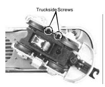
Figure 8. Screws to Remove to Access the Traction Tires
