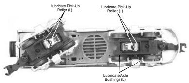
Figure 6. Lubrication Points on the Engine
