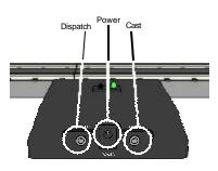
Fig.4: Overview of the Inputs on the Remote Lock On
