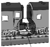
Push Down on Coupler Finger to Release Knuckle Figure 2. Coupling the Passenger Cars Together
