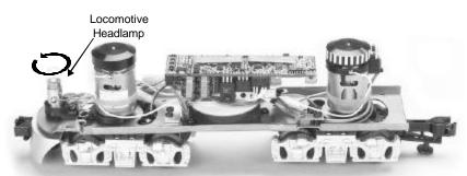
Figure 9. Location of the headlamp in the Engine.
