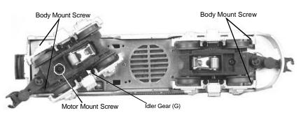
Figure 7. Body Mount Screws and Greasing Points.
