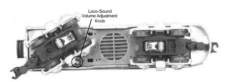
Figure 5. Location of the Loco-Sound Volume Adjustment Knob
