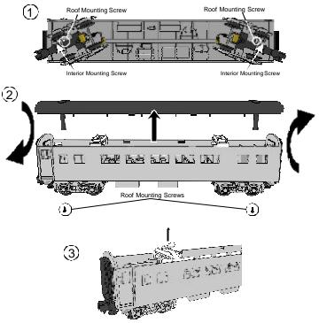
Figure 10. Instructions for Replacing the Lights in the Passenger cars.
