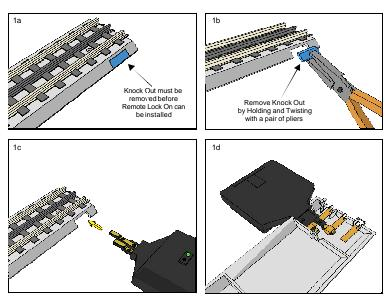
Fig. 1a-1d: Installation of Remote Lock On
