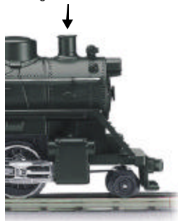
Figure 4. Add Smoke Fluid Through the Smoke Stack
