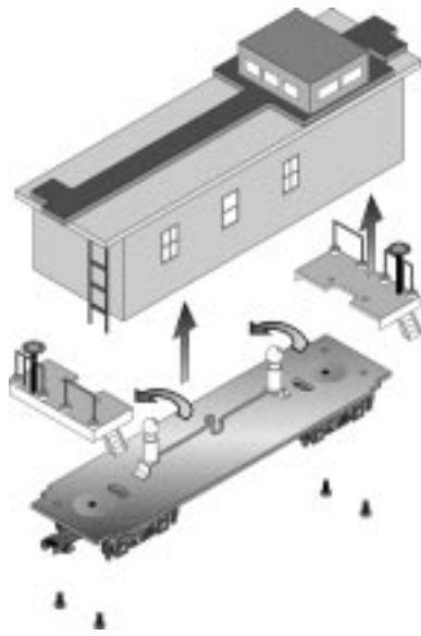
Figure 17: Removing the caboose body from its chassis.
