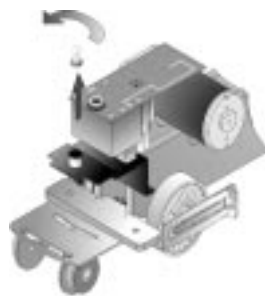
Figure 16: Locating and removing the light bulb.
