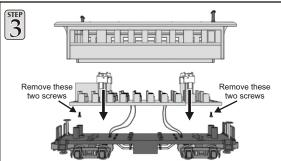
3) To be able to separate the interior from the shell you need to remove the screws from underneath the interior. With the two screws removed you can then lower the interior down from the shell.
