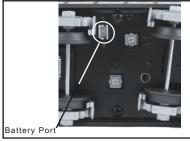
• Use M.T.H.'s battery recharger (Item No. 50-1019) (sold separately) that plugs into a wall outlet and a special port under the engine to recharge the battery overnight without leaving it on the track.
