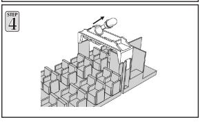
4) You can now replace the bulbs by pushing the socket up from the bulb holder and pull the bulb from its socket. Replace with a new one, and reverse the steps to reassemble the caboose.
