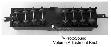
Figure 6: Adjusting The ProtoSound® Volume
