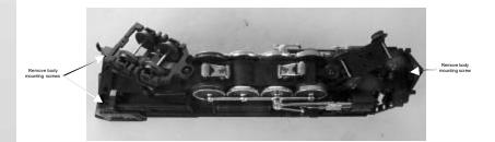
Figure 10: Removing The Boiler From The Chassis
