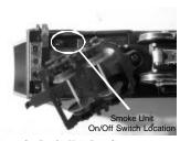
Figure 3: Smoke Unit Switch
