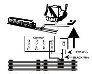
Figure 7: Wiring Up A Bell Button
