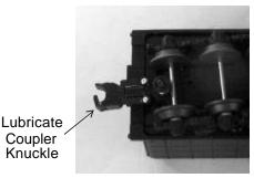
Figure 5: Lubricating The ProtoCouplers
