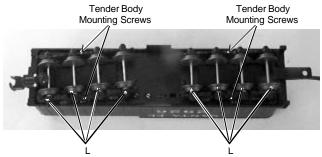
Figure 9: Lubricate The Tender Chassis Trucks
