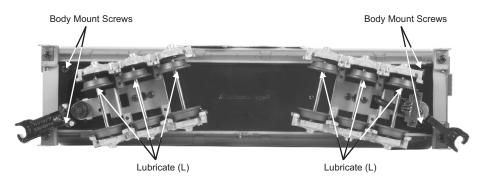
Figure 4. Auxiliary Tender lubrication points and body mount screws
