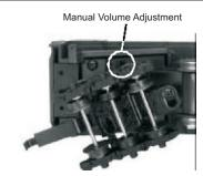
Figure 1. Proto-Sound 2.0 Volume Adjustment Knob
