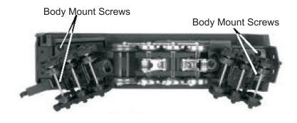
Figure 3. Greasing Points on the Engine and the Location of Body Mounting Screws
