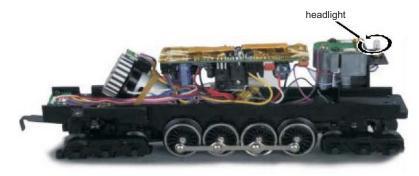
Figure 7. Replacing the Headlight
