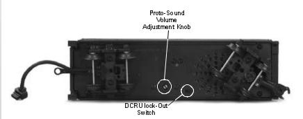
Figure 6: Adjusting The Proto-Sound® Volume
