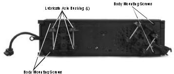
Figure 9: Lubricate The Tender Chassis Trucks
