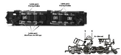
Figure 8: Lubricating The Locomotive Chassis
