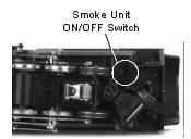
Figure 3: Smoke Unit Switch
