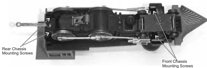
Figure 10: Removing The Boiler From The Chassis
