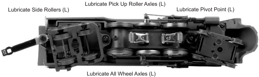
Fig. 1: Lubricating the Locomotive
