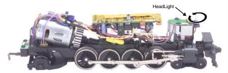
Figure 7. Replacing the Headlight
