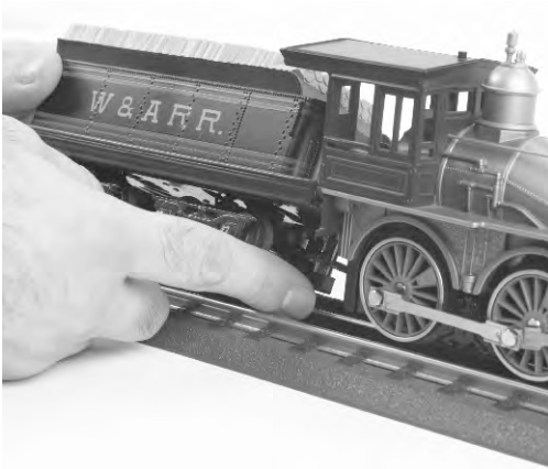
Figure: Attaching the Plastic Drawbar Holder
