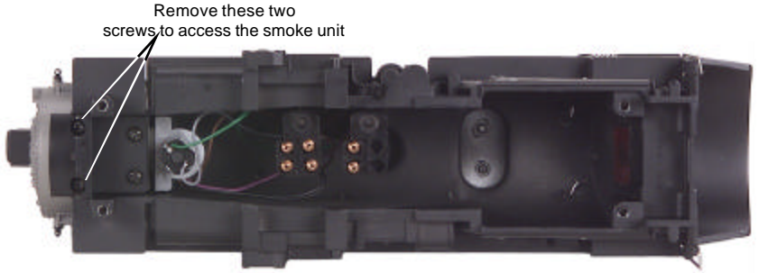
Figure 7. Removing the Smoke Unit Mounting Plate to Access the Smoke Unit
