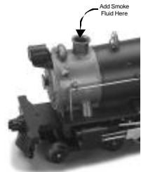
Figure 4. Add Smoke Fluid Through the Smoke Stack
