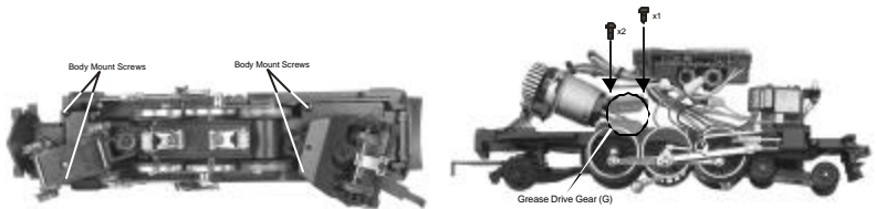
Figure 3. Locations of Body Mount Screws and Diagram for Greasing the Drive Gear
