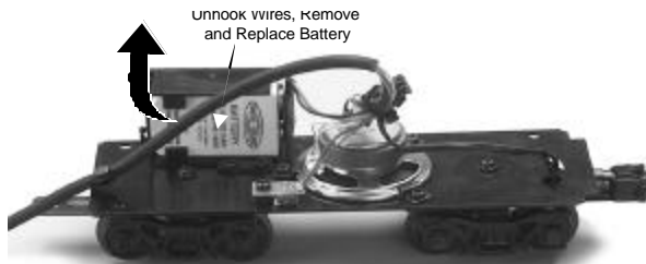
Figure 8. Unhook the Battery Leads, Remove the Battery and Replace with a New One.
