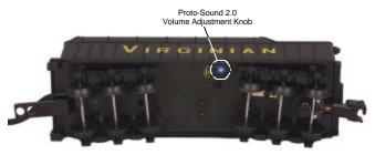
Figure 1. Proto-Sound 2.0 Volume Adjustment Knob
