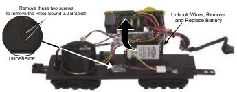
Figure 9. In order to easily get to the battery, temporarily remove the Proto-Sound 2.0 Boards by removing the two screws in the bottom of the tender. Replace the Battery, and reassemble in reverse.
