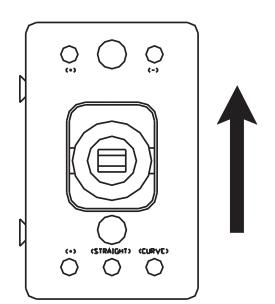
Push the remote switch lever toward the transformer lead wires to align the switch points to the curved direction.
