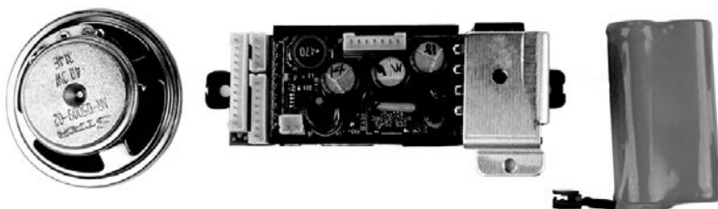
Typical component arrangement on tender floor. Note position of heat sink.
