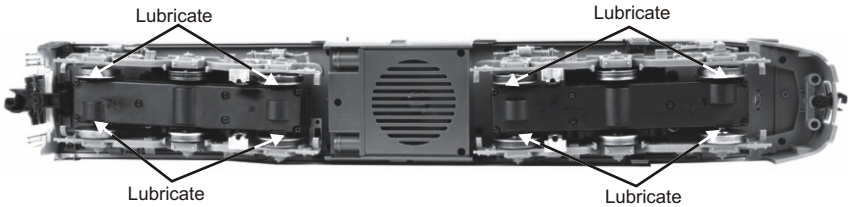
Lubrication Points on the Locomotive
