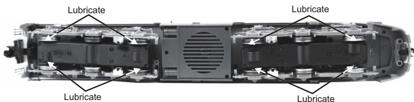
Lubrication Points on the Locomotive
