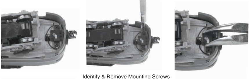
Identify & Remove Mounting Screws
