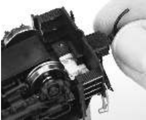
Line Up CENTER Mounting Hole In Coupler Pocket With Mounting Hole On Chassis
