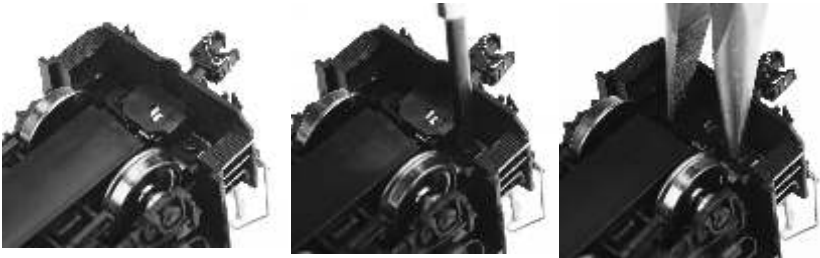
Identify & Remove Mounting Screws
