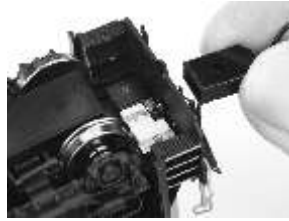
Insert Coupler Into Pilot (Shown Upside DOWN)
