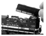
To remove the Control Hatch, gently pull it outward and lift it off from the side.
